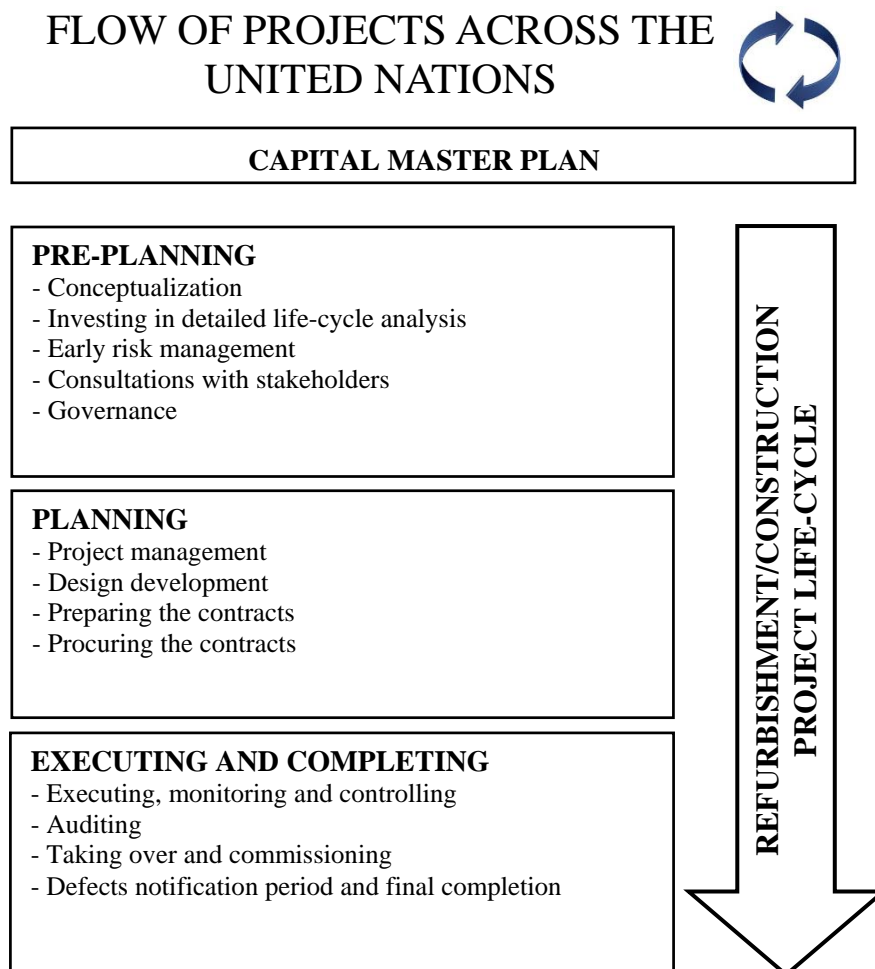
Chart 1. Capital/refurbishment/construction project's conception and flow
